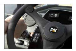
**Optional Auto-Shift Transmission** Work faster with the optional Auto-Shift transmission. The Auto-Shift transmission provides automatic shifting between five forward and three reverse gears. There is no floor mounted shift lever, so the operator has more floor space and better access through the right hand door.
